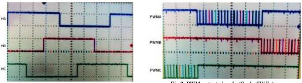
Fig.8. Motor Hall sensor signals. (Scale:5V/div)
