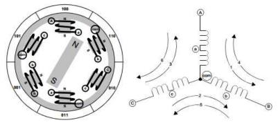
Fig.1 BLDC motor structure and stator winding
