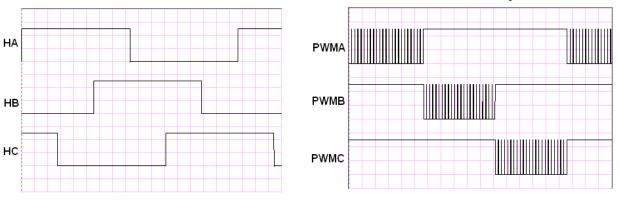
Fig. 5.Hall sensor signals(Scale:2V/div)
