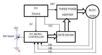
Fig.3. BLDC Motor Control System block diagram.
