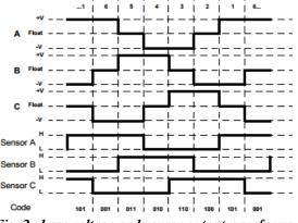
Fig. 2 phase voltage and sensor output waveforms.
