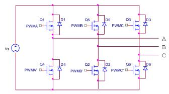
Fig. 4. Three phase Inverter Bridge
